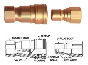
Gas-Mate couplings are one-way shut-off safety couplings designed for use with various fuel gases. Body sizes are 3/8", 1/2", 3/4", 1" and 1-1/4".
