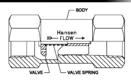
Series FS Flow Sensors are designed to protect personnel and property in case of hose failure in compliance with Federal Safety Regulations. Flow Sensors are intended for use with compressed air.
