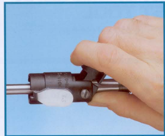
Cam lock compresses seal around O.D. of tube.
