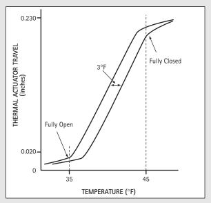
The limited hysteresis of the wax during changes in state from solid to liquid results in a narrow temperature dead band, providing very close control around the temperature set point.
