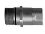
The Series 96 coupling is a heavy-duty wing nut coupling designed for use in hydraulic lines where dry break and minimum air inclusion are required. It is ideal for hydraulic dump trucks, oil field equipment, spreading equipment and applications requiring the ability to connect and/or disconnect under pressure. Body sizes are 3/4", 1" and 11/4".
